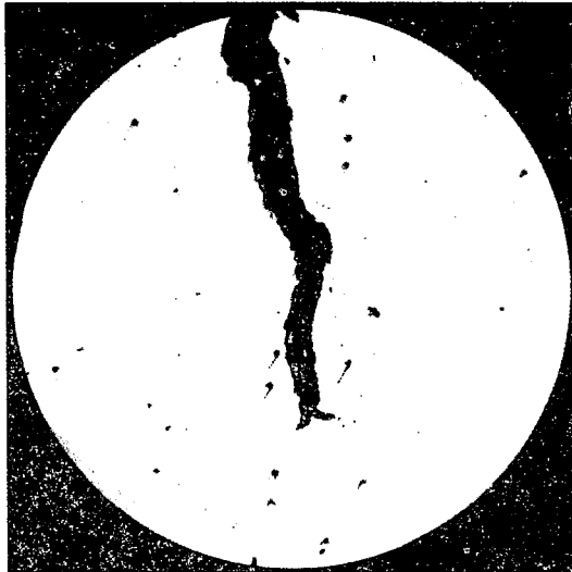
(B) A PHOTO-MICROGRAPH OF THE SAME FISSURE TAKEN AT THE POINT 5 IN PLATE X (A) WITH A MAGNIFICATION OF 250 DIAMETERS Here the fissure is still wider but less deep
